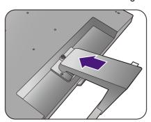
Tighten the screw(s) that fixes the stand to the monitor.
